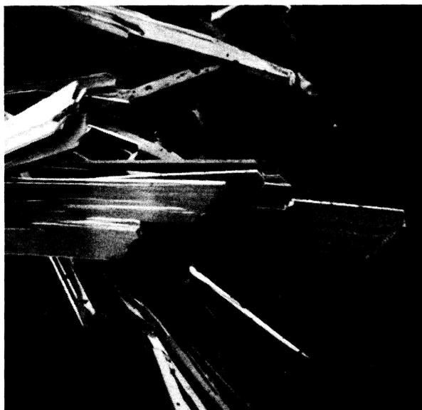
Fig. 1. Scanning electron microscope photomicrograph of ajoite showing the bladed habit. The width of the large crystal is about 0.1 mm.
