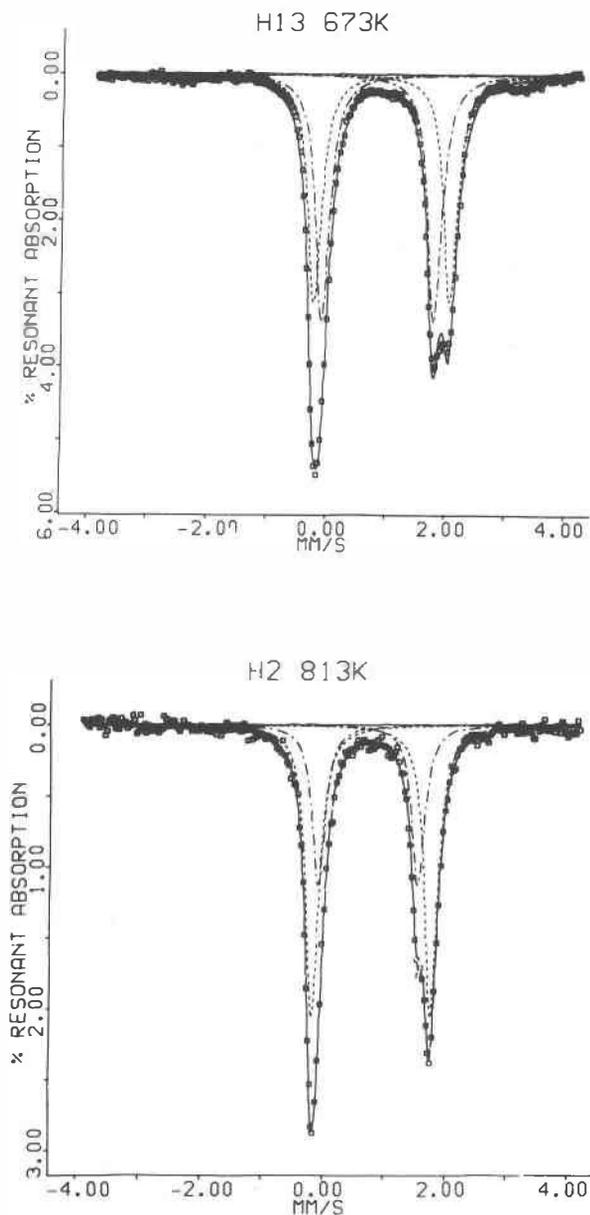
Fig. 1. Mössbauer spectra of the olivines H13 (above) and H2 (below) at elevated temperatures. Outer doublet (----) due to  $\text{Fe}^{2+}$  in the M2 site, inner doublet (- · -) due to  $\text{Fe}^{2+}$  in the M1 site.
