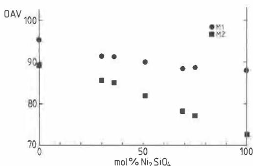
Fig. 4. Variation of the octahedral distortion parameter, OAV, with composition (see Table 7 for definitions).
