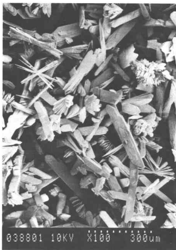
Fig. 1. Scanning electron micrograph of synthetic krautite.
