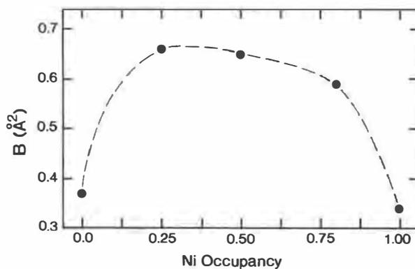
Fig. 3. Variation in M(1)-site isotropic displacement factors ( $B$ ) with Ni occupancy at the M(1) site. M(1) occupancies were fixed at nominal values; all other structural and pattern parameters [except M(1) displacement factors] were fixed at values from the final overall refinements.
