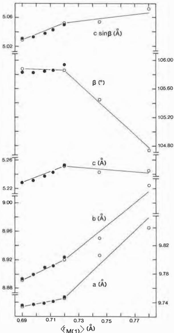
Fig. 4. Variation in cell parameters  $a$ ,  $b$ ,  $c$ ,  $\beta$  and  $c \sin \beta$  with mean ionic radius of the constituent cations at the M(1) site (solid circles). Open circles are data from the single-crystal structures of  $\text{CaNiSi}_2\text{O}_6$  and  $\text{CaCoSi}_2\text{O}_6$  (Ghose et al., 1987), diopside (Levien and Prewitt, 1981), and hedenbergite (Clark et al., 1969).
