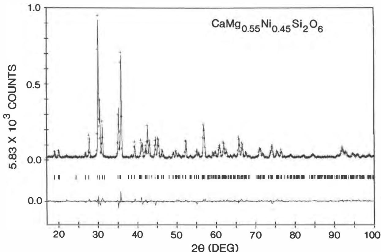
Fig. 1. Observed and calculated X-ray powder diffraction pattern for sample Ni<sub>50</sub> (CaMg<sub>0.55</sub>Ni<sub>0.45</sub>Si<sub>2</sub>O<sub>6</sub>). The crosses are the observed data, the solid line is the calculated pattern, and the vertical bars mark all possible Bragg reflections ( $K\alpha_1$  and  $K\alpha_2$ ). The difference between the observed and calculated patterns is shown at the bottom.
