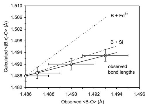
**FIGURE 8.** Calculated vs. observed mean bond lengths at T5 site. Open circles = experimental data (most symbols overlap). Solid line = linear regression. Dashed line = calculated <(B + Si) – O> distances. Dotted line = calculated <(B + Fe<sup>3+</sup>) – O> distances. Ionic radii from Shannon (1976).
