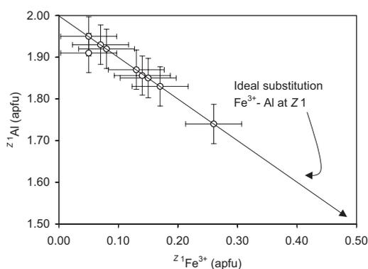
**FIGURE 7.** Populations of Al vs. Fe<sup>3+</sup> at Z1 site. Solid line, which represents ideal 1:1 substitution, coincides with linear regression of experimental data ( $r = 0.98$ ).
