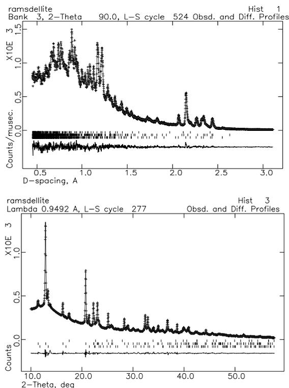
**FIGURE 3.** Final observed (crosses), calculated (solid line), and difference (lower) powder diffraction patterns for the Rietveld refinement of (a) ramsdellite and groutellite using powder neutron diffraction data, and (b) groutellite and ramsdellite using synchrotron X-ray diffraction data.
