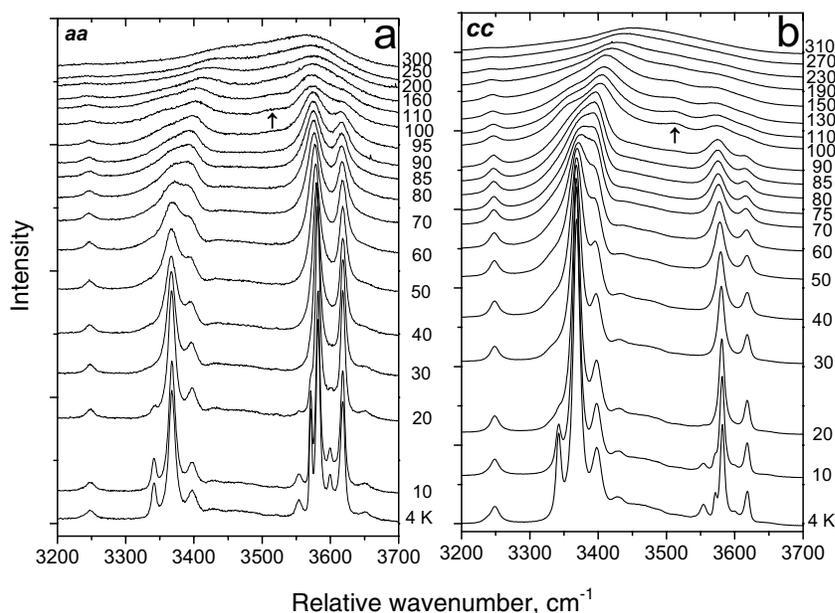
**FIGURE 5.** Temperature evolution of the polarized spectra showing the O-H and H<sub>2</sub>O stretching modes in hemimorphite; (a) *aa*-spectra and (b) *cc*-spectra. The appearance of the new band at around 3500 cm<sup>-1</sup> at  $T \geq 100$  K is shown by the arrow.
