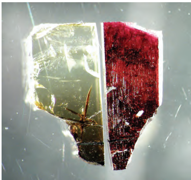
FIGURE 7. Unheated and heated (750 °C/30 h) piece of the same Mn-rich crystal (sample MNELB) from Elba Island, Italy. Both polished plates are ~8 mm in length and ~0.6 mm thick.
