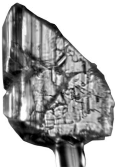
FIGURE 1. Tabular crystal of chromschiefelinite, 140 \times 110 \times 35 \mu\text{m} , used in optical and morphological studies. The crystal is tabular on {010} and striated parallel to [001]. Note that right side of the crystal is bounded by broken surfaces rather than faces.
