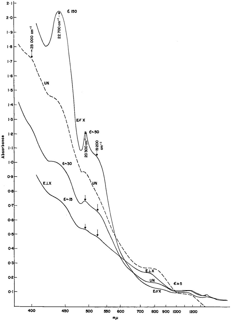
FIG. 1. Polarized and unpolarized (UN) spectra of transverse section of Old Chelsea phlogopite, thickness  $\sim 10^{-8}$  cm; UN—curve is that of a basal section.
