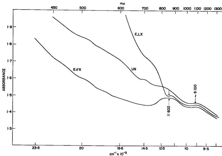
FIG. 2. Polarized and unpolarized (UN) spectra of a transverse section of Templeton phlogopite; thickness 0.056 cm.
