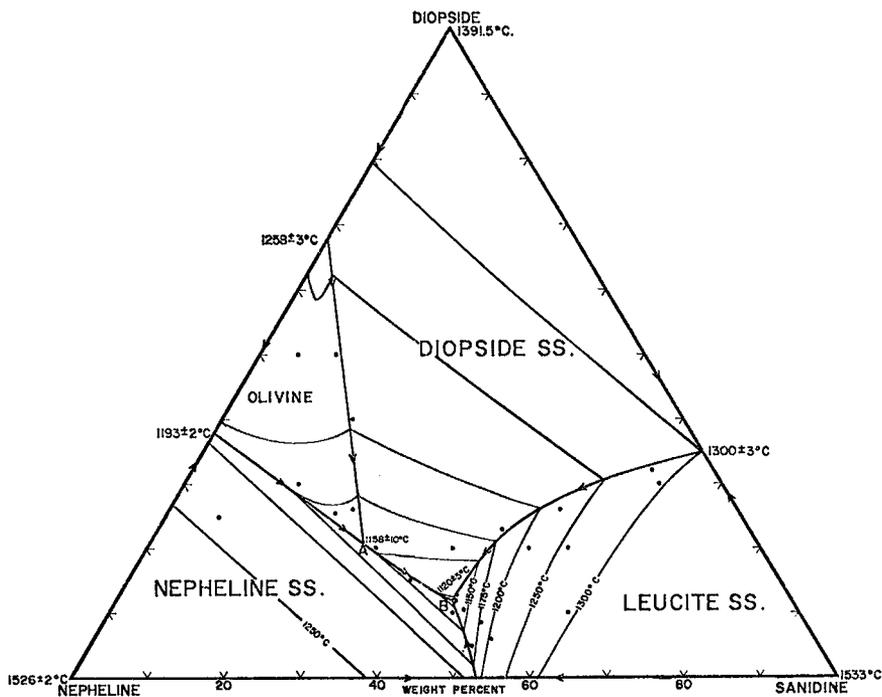
FIG. 2. Phase relations in the system diopside—nepheline—sanidine. Solid dots represent compositions in weight percent.
