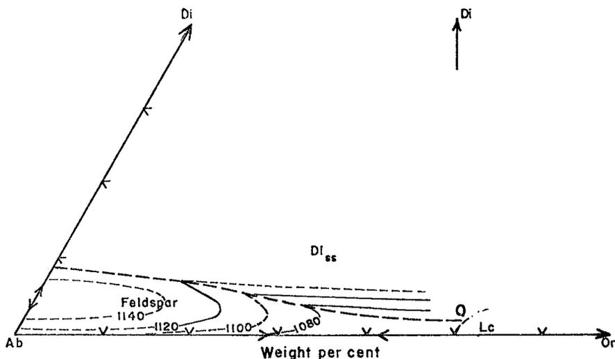
FIG. 4. Phase relations in the join diopside—albite—orthoclase, (after Morse 1968).
