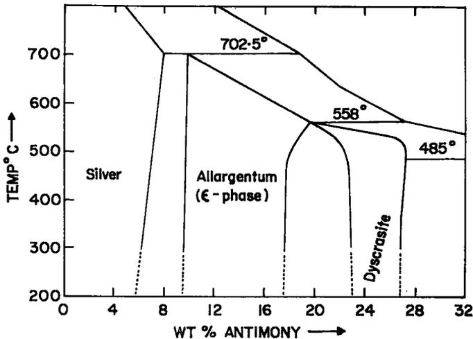
FIG. 124. Phase equilibrium diagram of the silver-rich end of the Ag-Sb system (From Somanchi 1966 and slightly modified by the authors).
