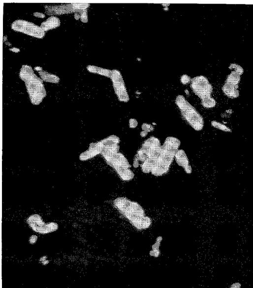
FIG. 1. Synthetic crystals of  $\text{Na}_2\text{Ca}_2\text{Sr}_2(\text{CO}_3)_5$ . Average length of crystals is approximately 0.03 mm.
