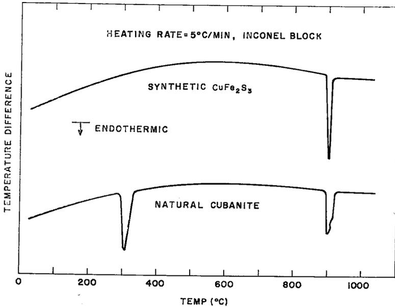
FIG. 1. — DTA curves for cubanite and synthetic  $\text{CuFe}_2\text{S}_3$ .
