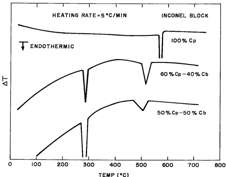
FIG. 6. — DTA curves for chalcopyrite-cubanite mixtures expressed in weight percentages.
