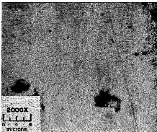
FIG. 3. — Photomicrograph of synthetic  $\text{CuFe}_2\text{S}_3$  heated to 800°C and then slowly cooled. Dark phase is retained *iss* and light phase is "chalcopyrite".
