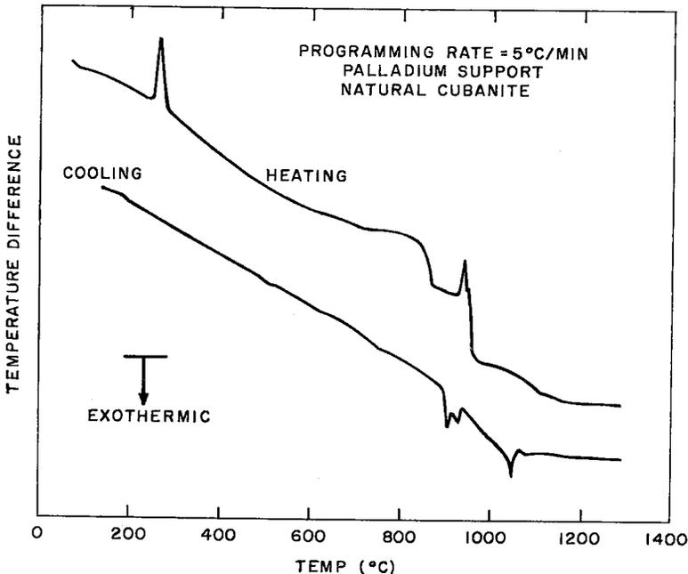
FIG. 2. — DTA curves obtained on heating and cooling for natural  $\text{CuFe}_2\text{S}_3$  (cubanite).
