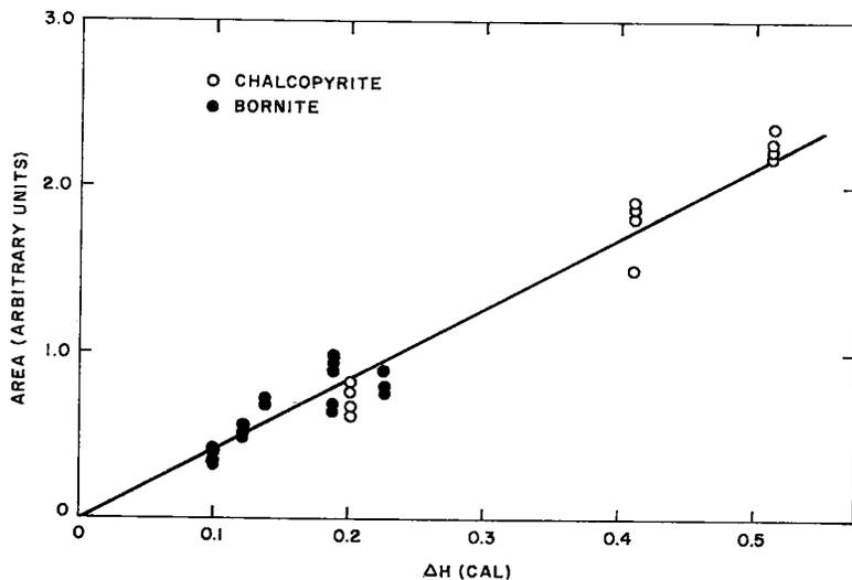
FIG. 4. — DTA calibration curve obtained for heating at 5°C/min with Inconel block.
