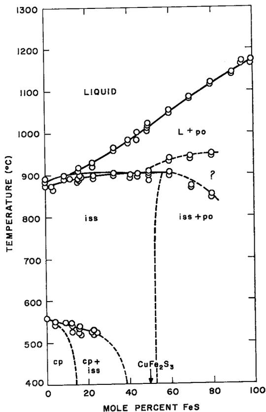
Fig. 7. — Partial phase diagram for the quasi-binary system  $\text{CuFeS}_2$ -FeS.
