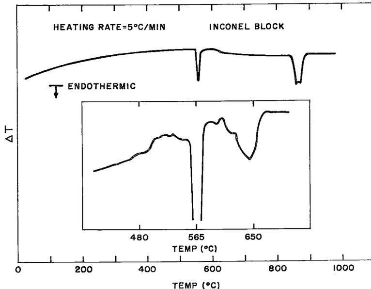
FIG. 5. — DTA curves for natural chalcopryrite.
