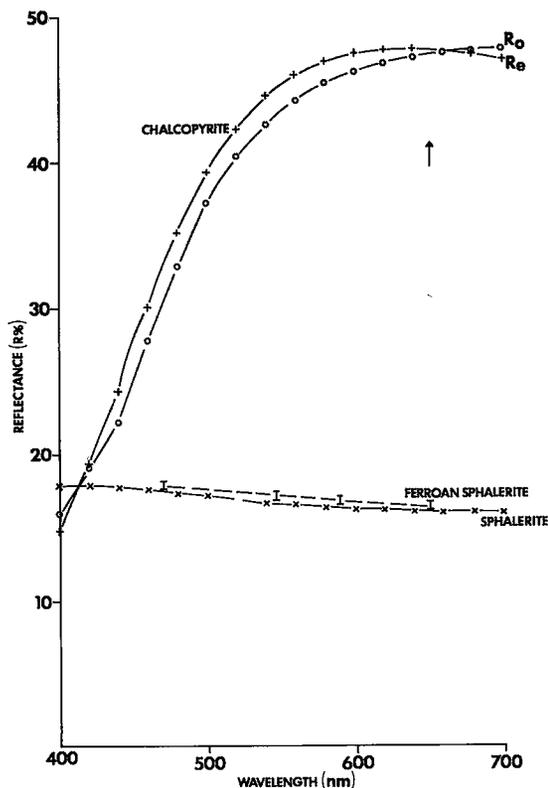
FIG. 2. Reflectance data for chalcopyrite, sphalerite and ferroan sphalerite in the visible region. Data from IMA/COM Data File (Henry 1977).
