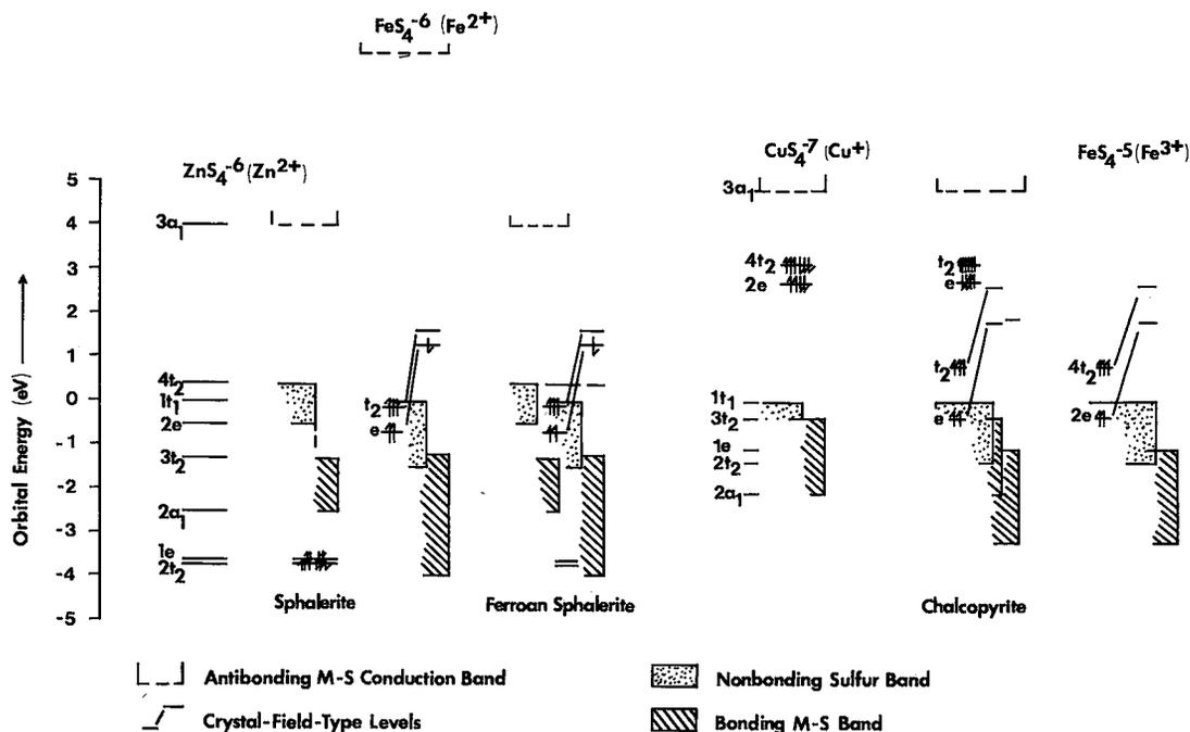
FIG. 1. Electron-structure models for sphalerite, ferroan sphalerite and chalcopyrite. Discrete energy levels are shown for clusters  $\text{ZnS}_4^{-6}$ ,  $\text{CuS}_4^{-7}$  and  $\text{FeS}_4^{-5}$  and composite "one-electron"-band model energy-level diagrams illustrated for the minerals.
