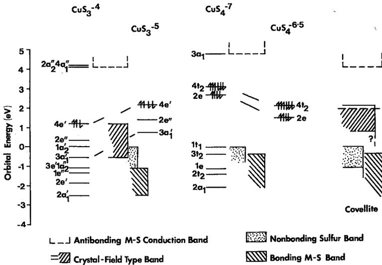
Fig. 3. Electron-structure model for covellite. Discrete energy-levels are shown for clusters  $\text{CuS}_3^{4-}$ ,  $\text{CuS}_3^{5-}$ ,  $\text{CuS}_4^{7-}$ ,  $\text{CuS}_4^{6.5-}$  and a composite "one-electron"-band model energy-level diagram illustrated for the mineral.
