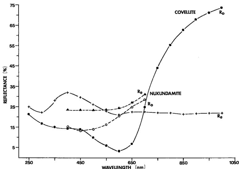
Fig. 4. Reflectance data for covellite and nukundamite. Data from IMA/COM Data File (Henry 1977) and Rice *et al.* (1979).
