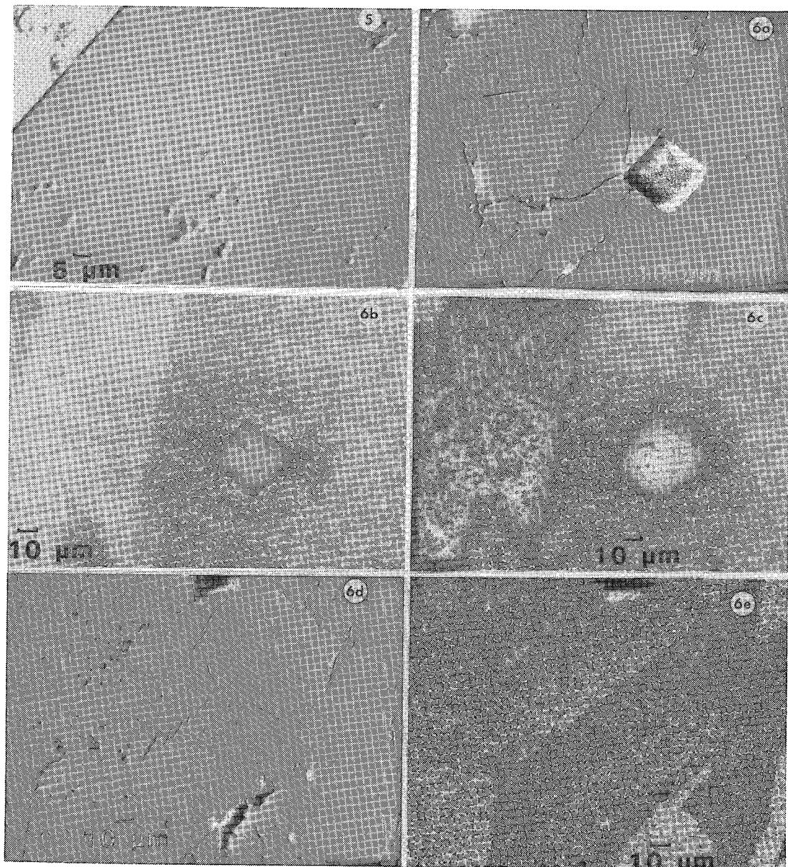
FIG. 5. Back-Scattered Electron (BSE) photograph of  $\text{Gal}_{60}\text{Mat}_{40}$  (medium grey) and host pyrite (white) from the Fairview mine, Round Mountain, Nevada. Sample DRS-73-228.
