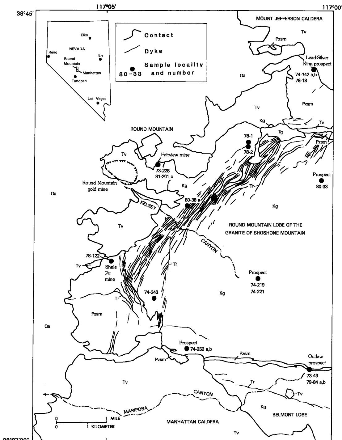
FIG. 1. Simplified geologic map of the Round Mountain quadrangle, showing locations of areas studied. Qa, Quaternary alluvium; Tv, Tertiary volcanic rocks (~24–27 Ma); Tg, Tertiary granodiorite stock (35 Ma); Tr, Tertiary rhyolite dykes (35 Ma); Kg, Cretaceous granite (~80–95 Ma); Pszm, Paleozoic sedimentary and metamorphic rocks.
