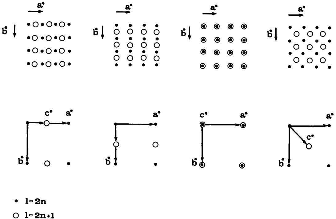
FIG. 4. The four kinds of diffraction patterns and the corresponding reciprocal unit-cells.
