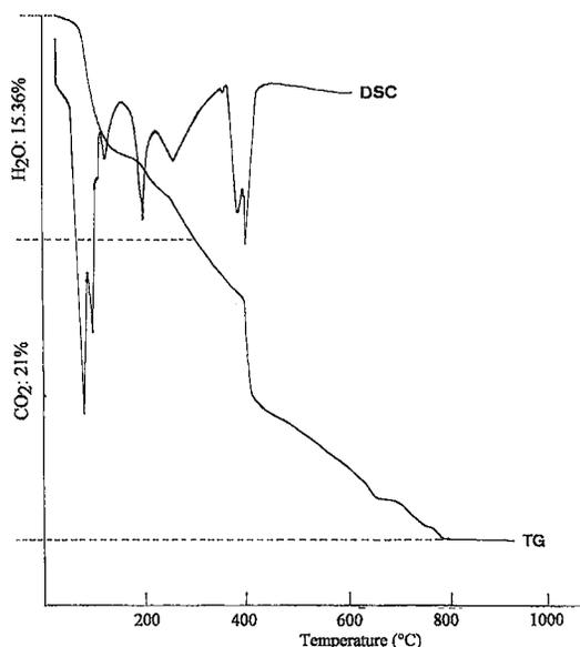
FIG. 2. Results of thermogravimetric (TG) and differential scanning calorimetry (DSC) analyses of the intermediate phase between liebigite and andersonite.
