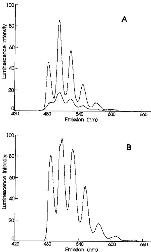
FIG. 3. Luminescence spectra of the intermediate phase between liebigite and andersonite. A. Fluorescence spectra at 77 and 298 K. B. Phosphorescence spectra at 77 K.
