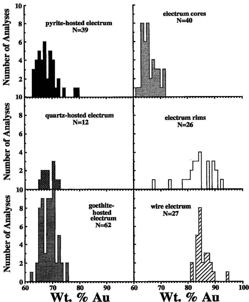
FIG. 2. Composition of the six types of electrum. Each datum represents the average composition for a given grain, core, rim or wire structures. N is the number of grains, rims or wires analyzed.
