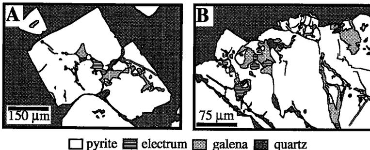
FIG. 3. Line drawings from photomicrographs illustrating the typical occurrence of pyrite-hosted electrum with galena in main-stage pyrite. A. Electrum and galena inclusions in pyrite. B. Electrum and galena along fractures in cataclastically deformed pyrite.
