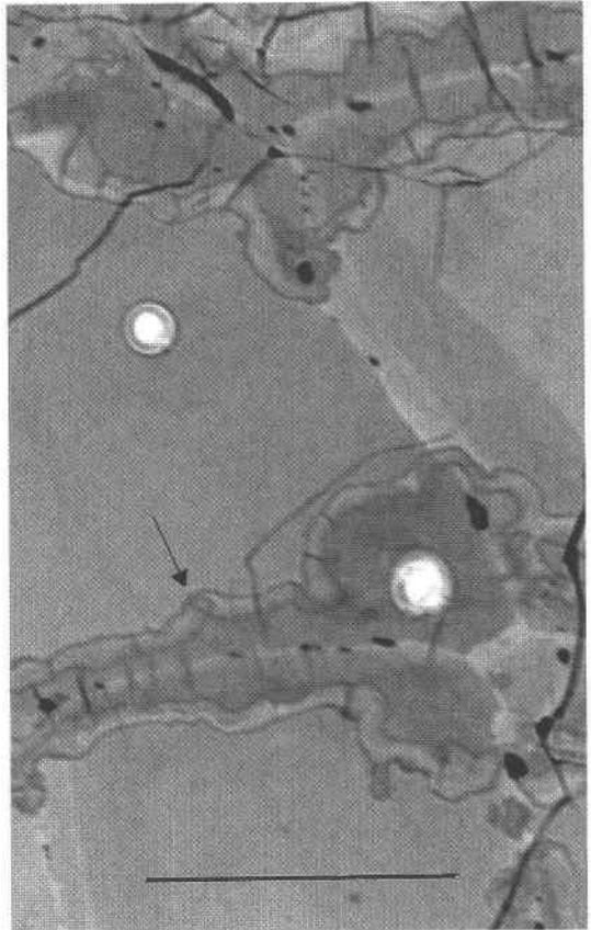
FIG. 6. Alteration fronts (seen as variations in grey level from dark to lighter grey) along polygon boundaries; younger alteration-fronts cross-cut older alteration-fronts (arrow). Apatite is still seen as anhedra (black) crystals concentrated along polygon boundaries. Fractures orthogonal to polygon boundaries are concentrated within altered margins. Scale bar is 20  $\mu$ m.
