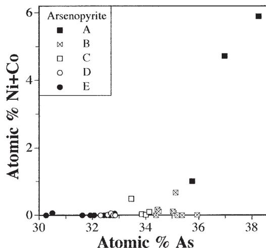
FIG. 3. The average content of Ni + Co (atomic %) and As (atomic %) in arsenopyrite from the samples studied. Note the very high Ni + Co content of arsenopyrite A.
