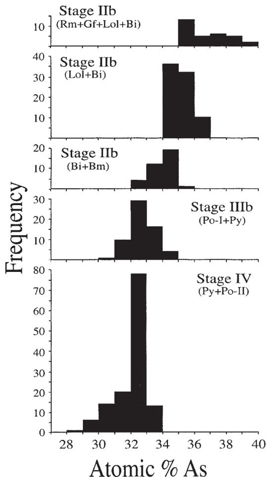
FIG. 5. Frequency distribution of As content (atomic %) in arsenopyrite of different stages and different assemblages from the Ulsan mine. See Table 1 for mineral abbreviations.
