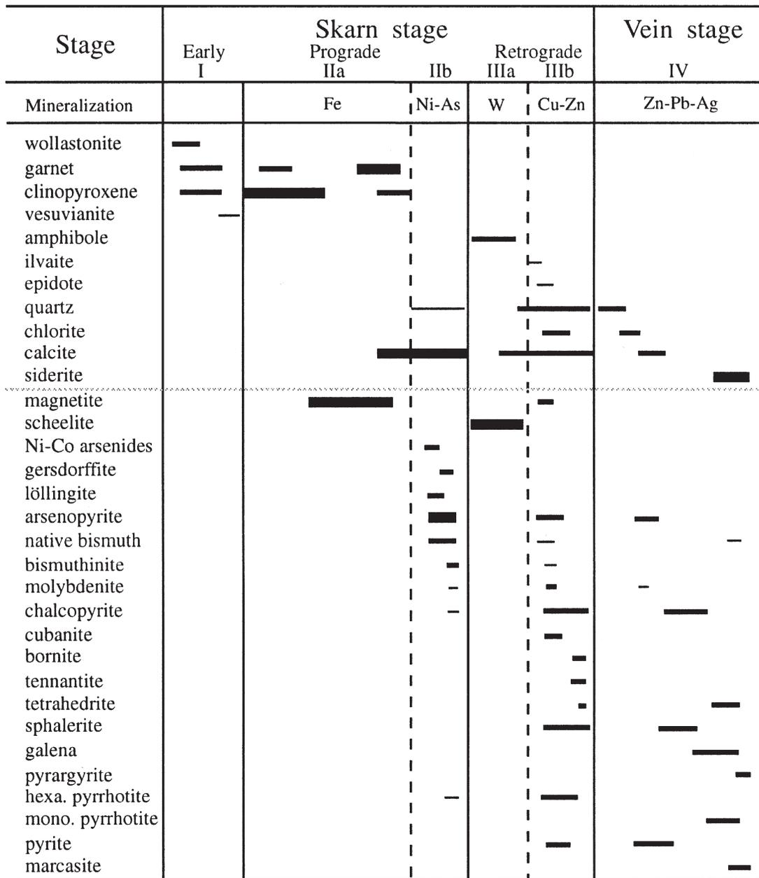
Fig. 2. Simplified paragenetic sequences for the assemblages of principal ore and alteration minerals at Ulsan mine. Line thicknesses represent schematically the relative abundances of the mineral deposited.
