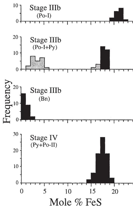
FIG. 6. Frequency distribution of FeS contents (mole %) in sphalerite of different stages and different assemblages from the Ulsan mine. Note the gap (shaded area) of FeS content (mole %) in sphalerite from specimen no. U820880 in stage IIIb (Po-I + py). See Table 1 for mineral abbreviations.
