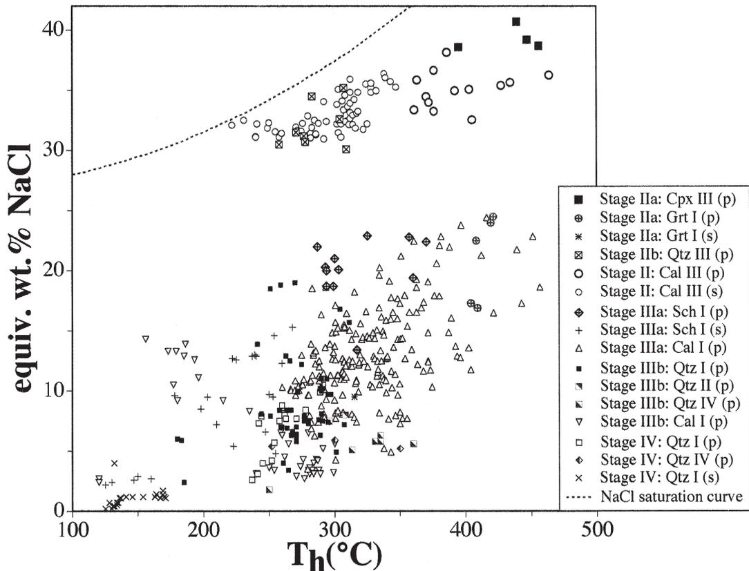
FIG. 10. Plot of homogenization temperature ( $T_h$ ) versus salinity (equiv. wt.% NaCl) for fluid inclusions in minerals from various stages of mineralization. Stages I, II, III and IV following mineral names are types of fluid inclusions. See Figure 8 for mineral abbreviations; p: primary, s: secondary.
