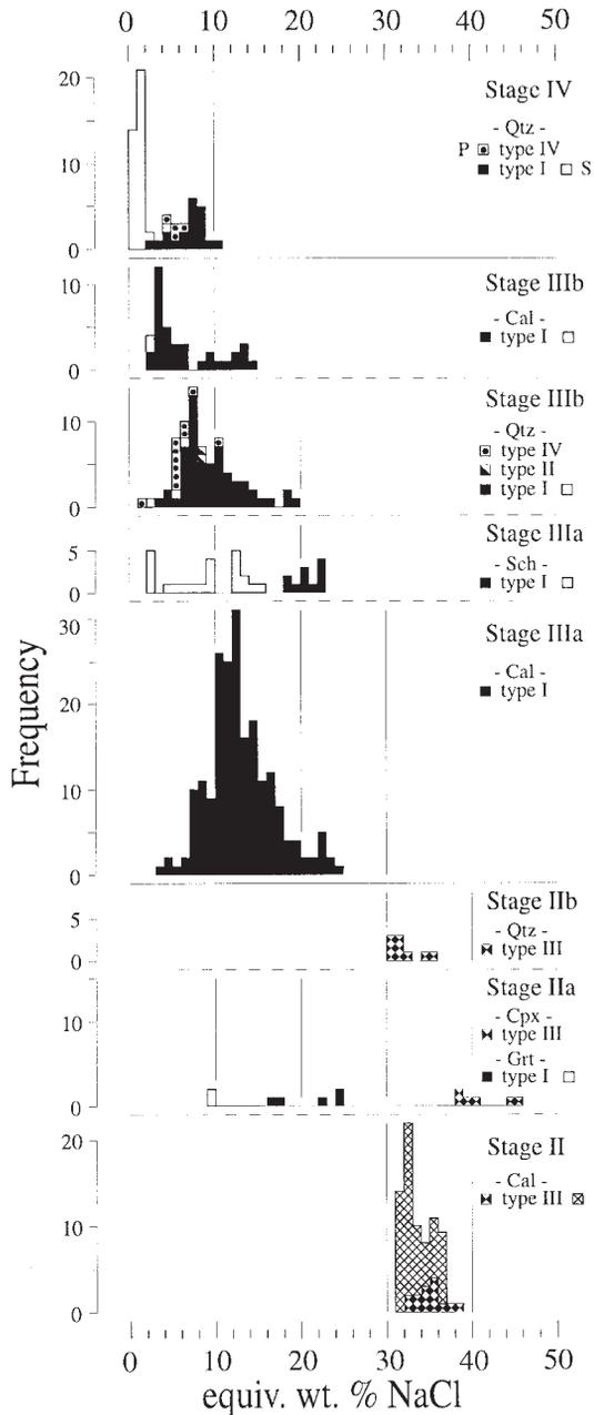
Fig. 9. Frequency histogram of salinity (equiv. wt.% NaCl) for fluid inclusions in skarn and vein minerals of the Ulsan mine. See Figure 8 for mineral abbreviations.
