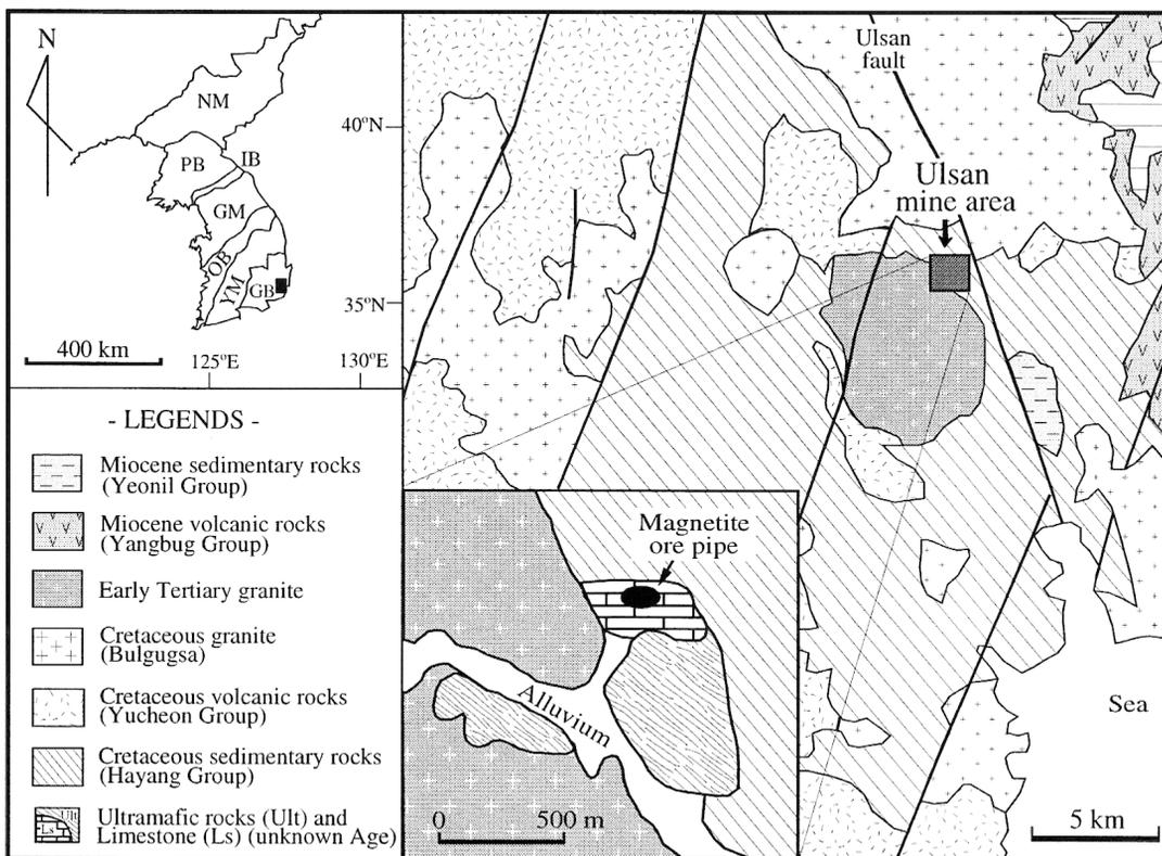
FIG. 1. Geological map of the Ulsan mine area showing the detailed map of the mining geology. The location of the Ulsan mine area (shaded box) is shown on the inset map of the Republic of Korea. GB: Gyeongsang Basin, GM: Gyeonggi Massif, IB: Imjingang Belt, NM: Nangrim Massif, OB: Ogcheon Belt, PB: Pyongnam Basin, YM: Yeongnam Massif.
