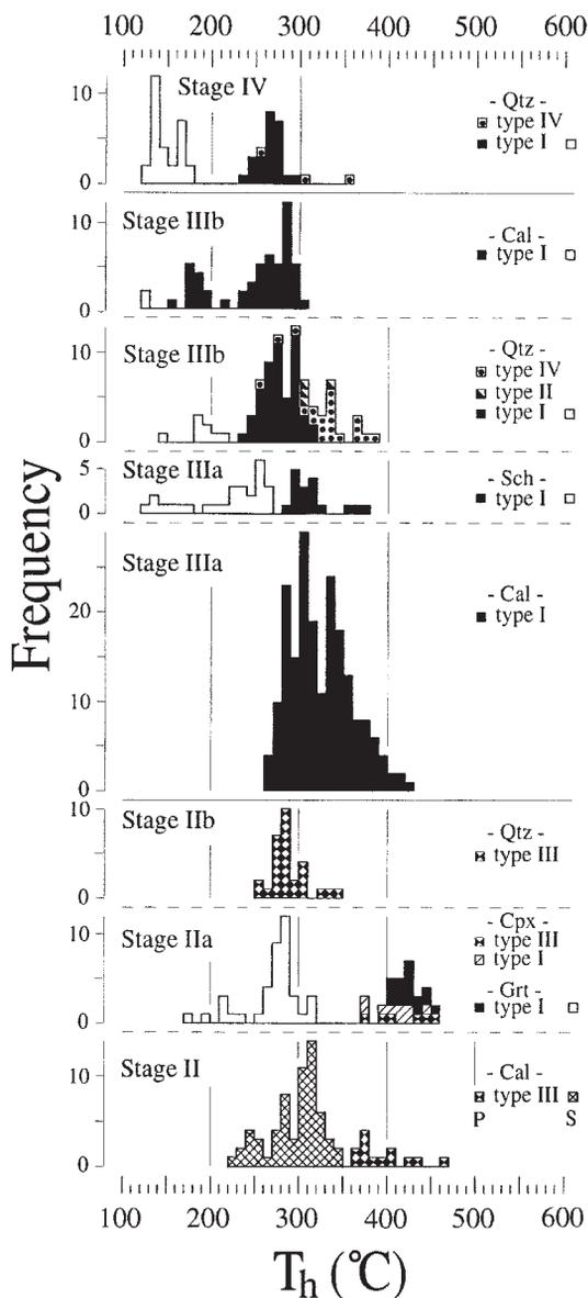
Fig. 8. Frequency histogram of total homogenization temperatures ( $T_h$ ) for fluid inclusions in skarn and vein minerals from the Ulsan mine. For type-IV fluid inclusions, decrepitation temperatures before anticipated homogenization are used as minimum estimates of homogenization. Cal: calcite, Cpx: clinopyroxene, Grt: garnet, Qtz: quartz, and Sch: scheelite.
