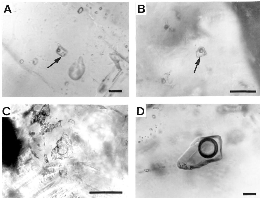
FIG. 7. Photomicrographs showing the types and occurrences of fluid inclusions in skarn and vein minerals from the Ulsan deposits. (A) Type-III hypersaline inclusion in stage-II calcite. (B) Type-III inclusion in stage-II clinopyroxene. (C) Type-I aqueous inclusion in stage-II garnet. (D) Type-IV CO<sub>2</sub>-bearing inclusion in stage-III quartz. All scale bars are 25 µm. Arrows point to halite as a daughter mineral in type-III inclusions.
