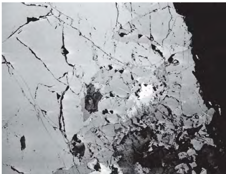
FIG. 4. Back-scattered electron image of bismutotantalite – stibian bismutotantalite; greyish white: native bismuth; pale grey: bismutotantalite; medium grey: stibian bismutotantalite; dark grey: microlite–bismutotantalite. Width of field of view: 1.1 mm.
