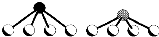
FIG. 1. The environments of the Pb and I sites in schwartzembergite; Pb site is a black circle, O atoms are high-lighted circles, I atom is a cross-hatched circle.
