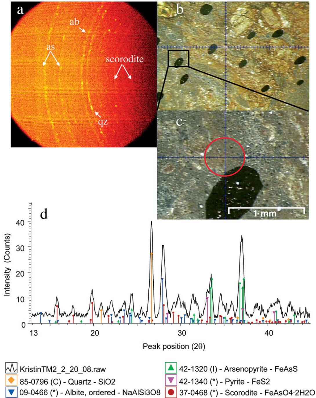
FIG. 4.  $\mu$ XRD pattern of scorodite aggregates (Type 1) containing silicate and sulfide inclusions: a) GADDS image with phases indicated on image, b) minimum zoom (field of view: 13 cm), with sample located inside black box, c) maximum zoom (field of view: 2 mm), with X-ray beam diameter (500  $\mu$ m) indicated by red circle, centered at crosshairs (collection time: 8 minutes), d) intensity *versus*  $2\theta$  plot, indicating matching phases.
