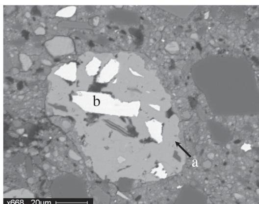
FIG. 2. Back-scattered electron image (SEM) of transition-zone material from the core, featuring: Type-1 iron arsenate (a), containing inclusions of weakly altered arsenopyrite (b).
