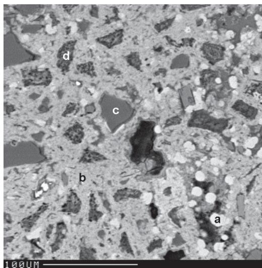
FIG. 3. Back-scattered electron image (SEM) of highly altered material from the bucket, featuring: primary Type-2 iron arsenate inclusions (a), resistant sulfide grains (c), and remnants of highly altered sulfides grains (d) in a matrix of iron sulfo-arsenate (b).
