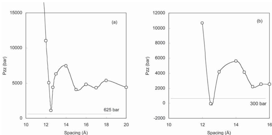
FIG. 6. Variation of the pressure tensor  $P_{zz}$  with the  $d_{001}$  value, grand canonical  $\mu$ VT ensemble, at (a) 353 K, 625 bar,  $-5.88$  kcal/mol (b) 333 K, 300 bar,  $-7.21$  kcal/mol. The horizontal bars correspond with the 625 and 300 bar pressures.
