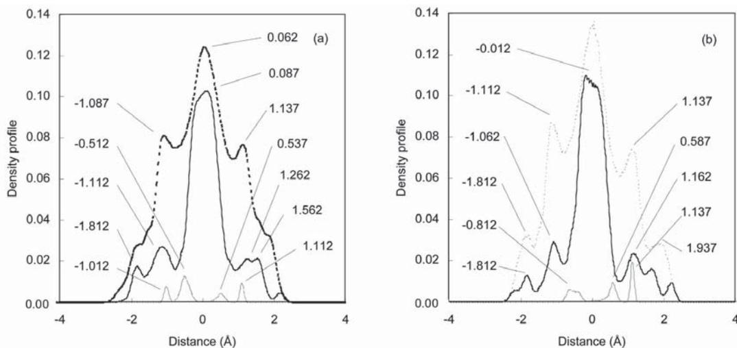
FIG. 7. Density profile of one-layer Ca-exchanged montmorillonite hydrate at (a) 353 K and 625 bar, (b) 333 K and 300 bar,  $\mu$ VT ensemble.
