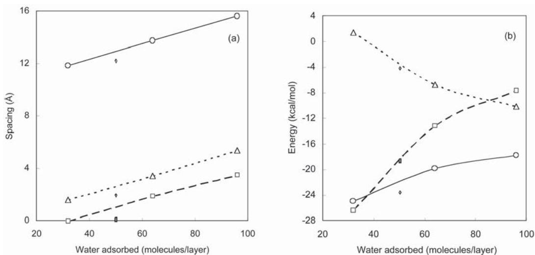
FIG. 4. Solvation of Ca-exchanged montmorillonite,  $\text{NP}_{\text{zzT}}$  ensemble, at 353 K and 625 bar. (a) Variation of the  $d_{001}$  value (o), outermost separation of  $\text{H}^+$  atoms ( $\Delta$ ),  $\text{O}^{2-}$  separation of  $\text{H}_2\text{O}$  molecules ( $\square$ ). (b) Variation of the internal energy (o), Coulomb contribution ( $\Delta$ ), and Lennard-Jones contribution ( $\square$ ). Small circles represent the same variables at 333 K and 300 bar.
