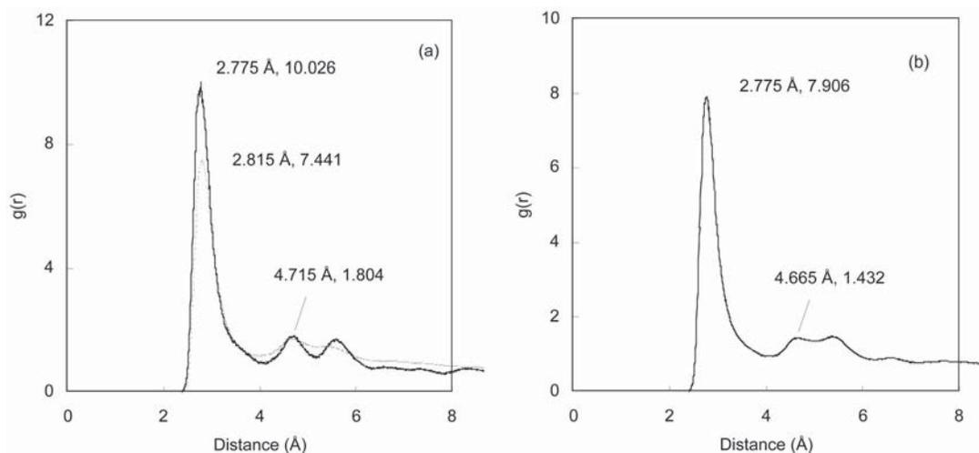
FIG. 3. Radial distribution function  $g_{\text{CaO}}(r)$  of hydrated Ca-exchanged montmorillonite at (a) 353 K and 625 bar, 32 (solid line) and 64 adsorbed molecules of  $\text{H}_2\text{O}$ ; (b) 333 K and 300 bar, 50 adsorbed molecules of  $\text{H}_2\text{O}$ .
