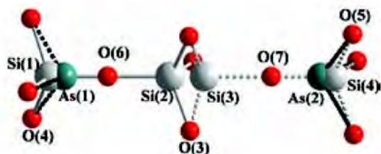
FIG. 1. A view of the two disordered orientations of the anions. The Si-O bonds in the \text{Si}_2\text{O}_7 group are shown in light gray, the \text{As}^{3+}\text{-O} bonds are represented in black. The bonds in the prevailing orientation are represented as solid lines.
