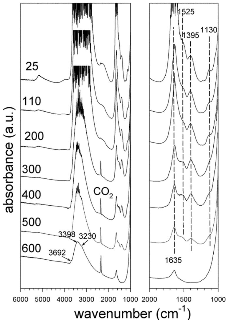
FIG. 4b. High-temperature FTIR spectra of yukonite from Grotta della Monaca. Temperature in  $^\circ\text{C}$ . On the left side, the  $2000\text{--}1000\text{ cm}^{-1}$  range is magnified for clarity.
