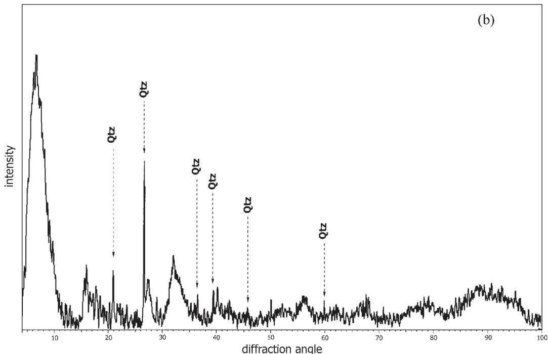
FIG. 6b. X-ray powder-diffraction patterns of yukonite from the Daulton mine with quartz.  $\text{CuK}\alpha_1$  radiation, Guinier geometry. The background has been subtracted, and diagrams have been smoothed.
