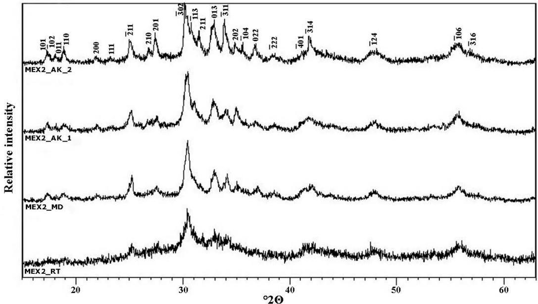
FIG. 2. XRD patterns of sample MEX2 at room temperature (MEX2\_RT) and heated in a microwave digester (MEX2\_MD) at 200–260°C for 20 minutes and in an autoclave at 150°C for 2 (MEX2\_AK\_1) and 5 h (MEX2\_AK\_2).
