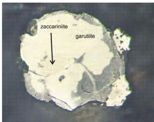
FIG. 2. Microphotograph (plane polarized reflected light, magnification 200 \times ) of zaccariniite in association with garutiite.
