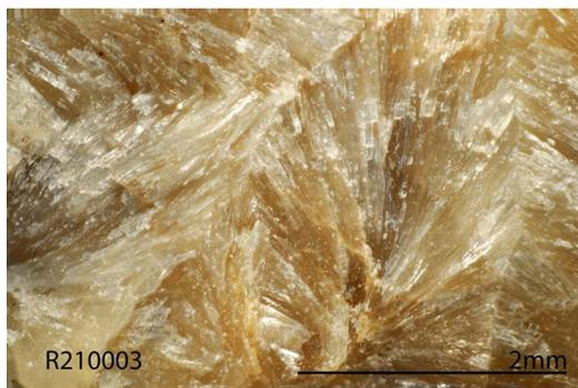
FIG. 2. A microscopic view of white to straw-yellow or tan radiating bladed crystals dondoellite.
