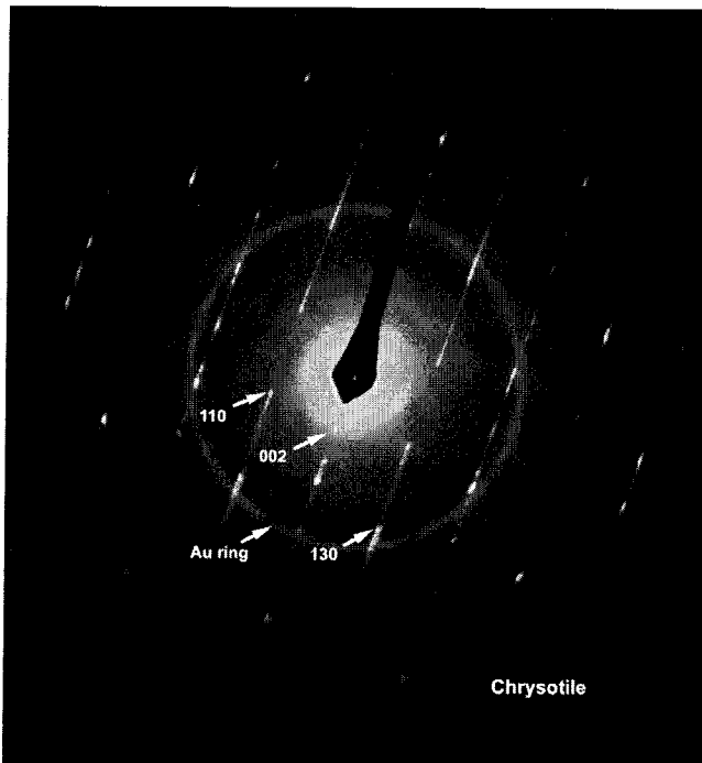
Figure 2.7 Chrysotile SAED pattern. The gold ring results from coating the fiber with a thin layer of gold and is used for calibration.
