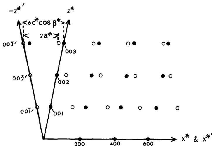
FIG. 2. One quadrant of the composite reciprocal lattice of the two components of a twinned amphibole approximating to amosite in cell parameters. Axes and indices of the second component of the twin (empty circles) are distinguished by primes from those of the first component (filled circles).
