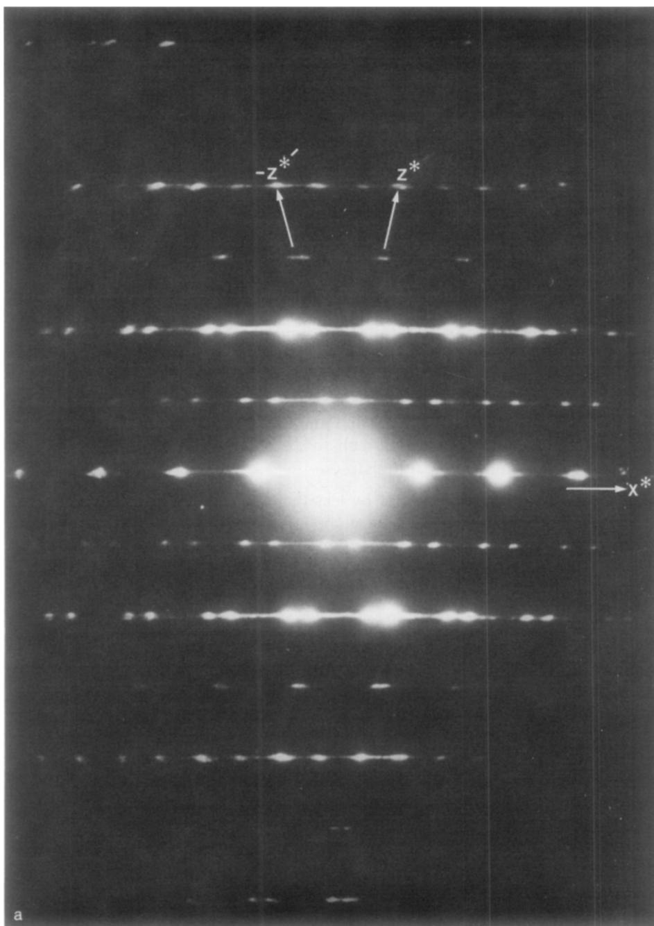
FIG. 1. Electron diffraction patterns with the beam parallel to  $[010]$ , and containing the  $h0l$  reflections: (a) amosite, (b) crocidolite. Both patterns show twinning on  $(100)$ . On the third-layer line the spots form much closer pairs on (a) than on (b). (Reproduced from *Acta Crystallographica*.)
