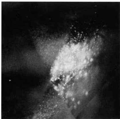
Figure 6. Reflections from plate-like inclusions (x25).
