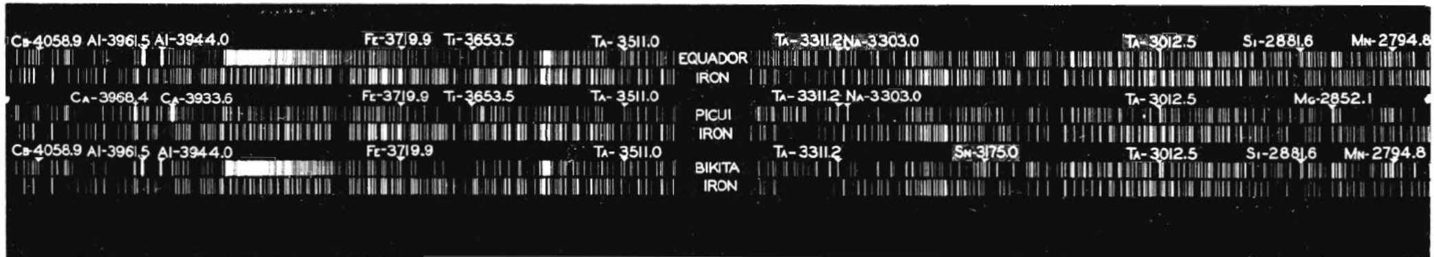
FIGURE 1. SPECTROGRAMS OF SIMPSONITE AND MICROLITE Iron lines are shown opposite each spectrogram for comparison. Photographs by Dr. W. M. Shafer.
