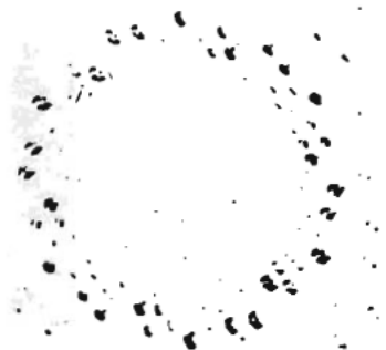
FIGURE 1. PRINT OF TAYLOR'S SIMPSONITE PHOTOGRAPHED NORMAL TO (0001)
