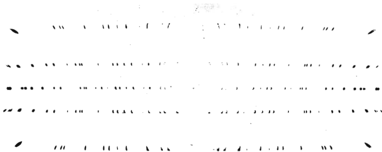
FIGURE 2. SIMPSONITE ROTATED ABOUT C-AXIS Spots are due to copper radiation filtered through nickel foil.
