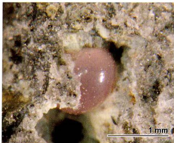
Figure 1 Photomicrographs of the spherical aggregate composed of kozoite-(La) and kozoite-(Nd).
