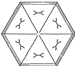
Fig. 2. Basal section of the Muiane cookeite showing twinning and optic axial plane.
