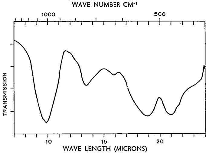
Fig. 3. Infra-red absorption spectrum of the Muiane cookeite.
