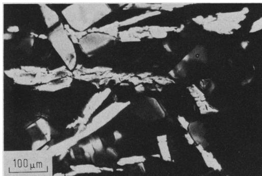
FIGS. 1 and 2. FIG. 1 (top). Photomicrograph of silica brick zone 4/1 ('hot' zone). Crossed nicols. FIG. 2 (bottom). Photomicrograph of silica brick zone 4/5 ('cold' zone). Crossed nicols.
