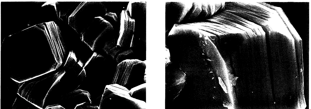
FIG. 2. Scanning electron micrographs of synthetic meta-uranocircite II crystals derived from chernikovite. Field width is 60 and 120 μm respectively. Field width is 60 μm (A, left) and 120 μm (B, detail of A, right).
