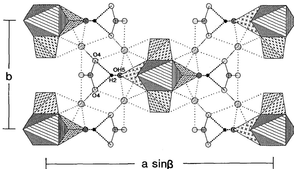
FIG. 3. The borcarite structure projected down the  $c$ -axis.  $B\phi_4$  tetrahedra are shaded with crosses,  $Mg\phi_6$  octahedra are ruled with parallel lines, oxygen atoms are stippled, OH anions are cross-hatched, C atoms are shaded with a herring-bone pattern, Ca atoms are ruled with broken parallel lines and H atoms are shown as small solid circles. Ca- $\phi$  bonds are dotted, C- $\phi$  are solid lines, H- $\phi$  bonds are broken lines.
