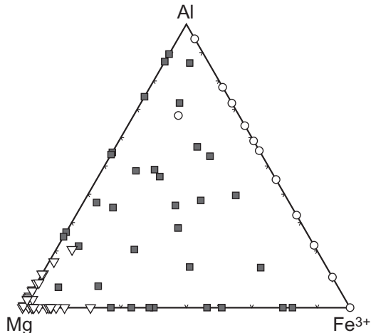
FIG. 6. A ternary plot showing the copiapite samples with a single phase of the type AL (open circles), single phase of the type MG (open inverted triangles) and samples with multiple copiapite phases (black squares). The plot shows the molar proportions of Mg, Al and Fe 3+ at the A site in the copiapite structure. Note that for the samples with multiple copiapite phases, only the total chemical composition could be plotted. Because of their fine-grained nature, we were not able to determine the composition of the co-existing phases.
