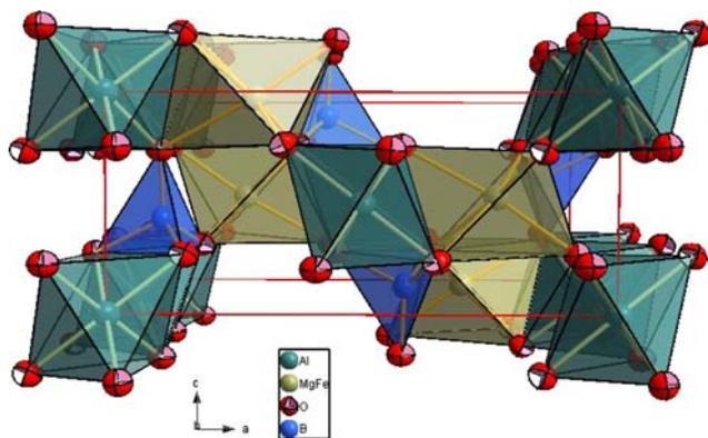
**Fig. 1** Polyhedral representation of the sinhalite structure based on the data of the structure refinement of the sinhalite sample from Hamburg, New Jersey (this work)
