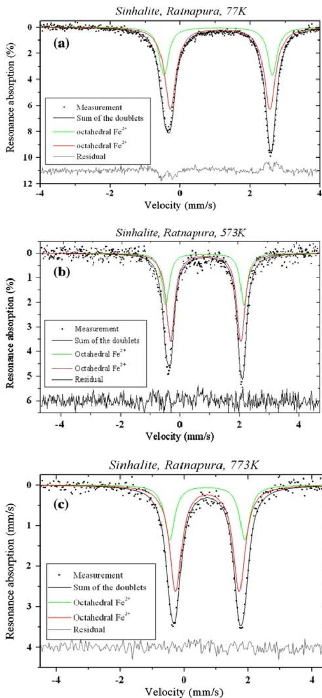
**Fig. 3** Mössbauer spectra of sinhalite from Ratnapura at 77 K (a), 573 K (b) and 773 K (c)
