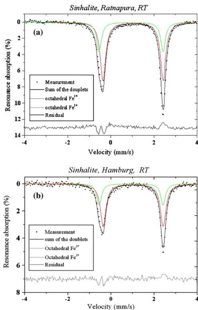
**Fig. 2** Mössbauer spectra of sinhalite from Ratnapura at 293 K (a), and from Hamburg, New Jersey at 293 K (b)
