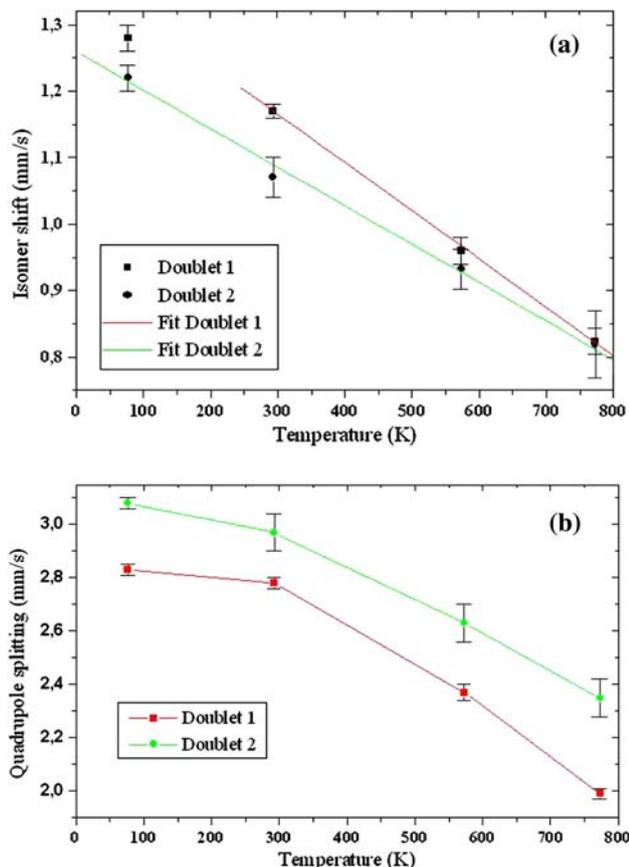
**Fig. 4** Temperature dependence of the isomer shift (a) and of the quadrupole splitting (b). In a the lines represent the result of a fitting procedure whereas in b the lines just connect the measured data
