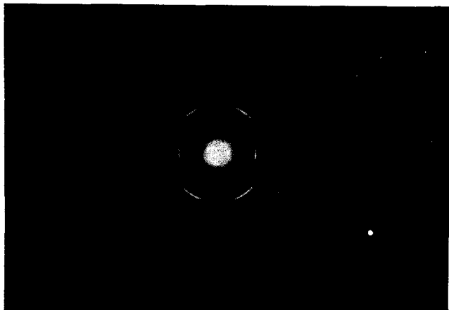
Fig. 2. Electron-diffraction pattern from selenium; the texture axis is [0001].
