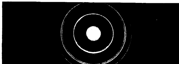
Fig. 2. Electron diffraction photograph from the polycrystalline aggregate of the cubic phase of \text{Cu}_3\text{SbS}_3 .
