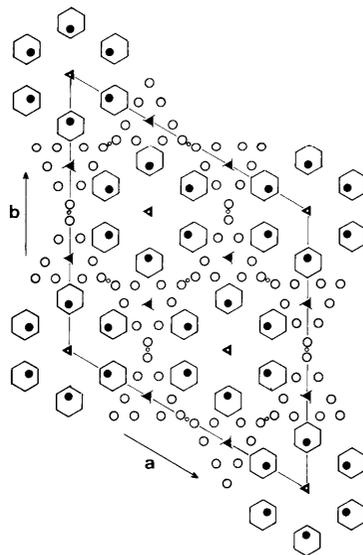
Fig. 3. Schematic projection of  $\text{BiNa}_3(\text{P}_3\text{O}_9)_2 \cdot 9\text{H}_2\text{O}$  down  $\bar{c}$ .  $\text{P}_3\text{O}_9$  rings are shown as hexagons. Empty and filled circles indicate Na and Bi atoms respectively. Water molecules are not represented.
